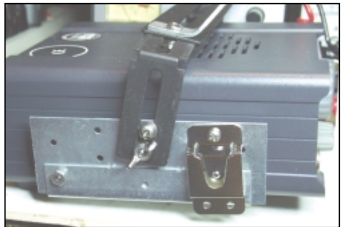
Photo 3— Details of the side attachments to the radio as well as the mounting of the top bracket and mic clip.
