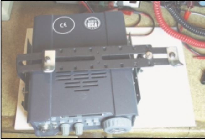
Photo 4— Once the mounting assembly is complete, it can be attached with wing nuts to a standard RadioShack bracket for mounting in your vehicle.
